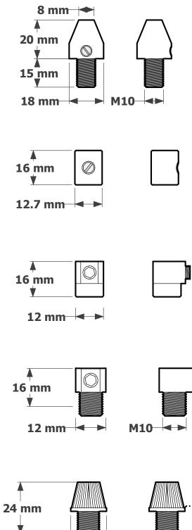
The **BRASS FEMALE CORD GRIP** can easily fit over the cable and keep it held into place with either a black or white plastic grub screw. Each end has an M10 internal thread allowing more options for it to be fitted. PRODUCT CODE 090-020-030
