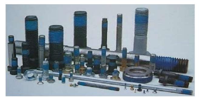
ELETTRA PRODUCTS has a process that can be applied to fasteners to provide a self-locking capability. The Elettra-Lok fused pad self-locking fasteners provide a permanent locking method into any tapped hole, especially where conditions involve vibration, shock, or adjustability, and is low cost relevant to similar self-locking techniques.
