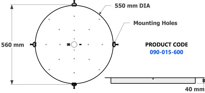
Every canopy is supplied with a mounting bracket. Ensure that the fixing screws are attached to the surface through each of the mounting holes.
