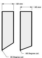
The metro six can be manufactured with a pencil cut, 45 degrees or 60 degrees, at the top and bottom or just one end of the fitting.
