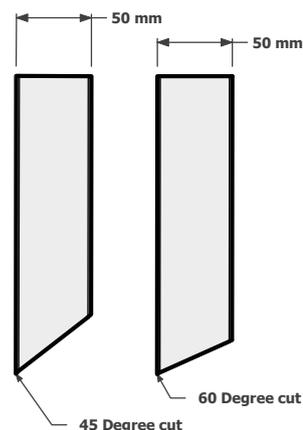
The metro five can be manufactured with a pencil cut, 45 degrees or 60 degrees, at the top and bottom or just one end of the fitting.
