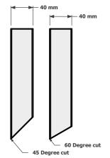
The metro four can be manufactured with a pencil cut, 45 degrees or 60 degrees, at the top or bottom or both ends of the fittings.
