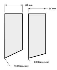
The Metro Eight can be manufactured with a pencil cut, 45 degrees or 60 degrees, at the top and bottom or just one end of the fitting.
